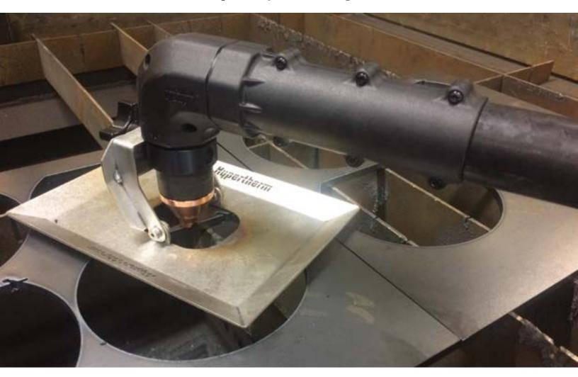
One of the most difficult jobs involved with mechanized cutting is dealing with the skeleton after removing cut parts. Skeletons can be heavy and unwieldy to handle, or flex unpredictably. Thin gauge material sometimes has a sharp edge that can lead to cuts even when the operator is wearing gloves. The Hypertherm Powermax® system and Duramax are the perfect combination to make clean up after mechanized cutting safer and faster, resulting in a more profitable operation.
